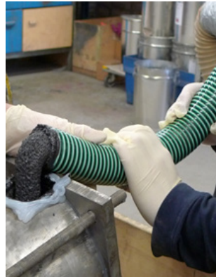
Polymer concrete casting process.
